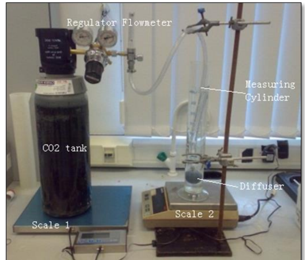
Figure 11 Experiment rig for carbon solidification process.
